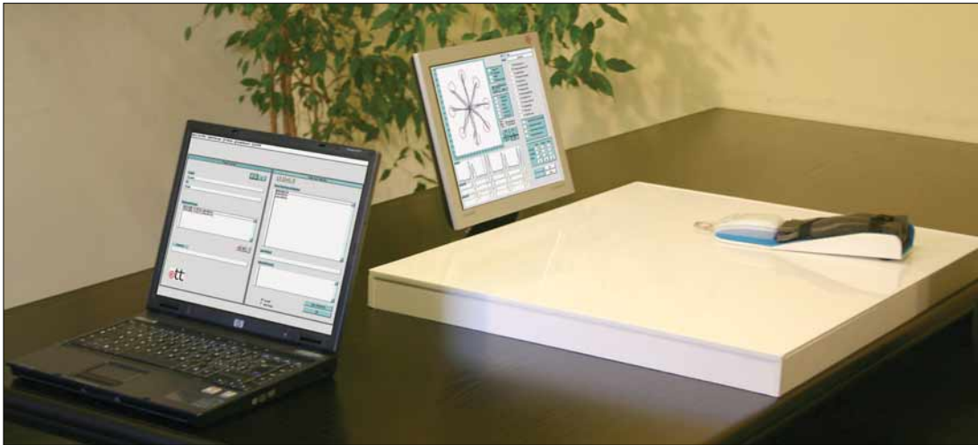
Figure 2: The figure shows the system: the laptop on the left let the doctor creates and selects the protocols, and supervises and analyses the subject performances; on the right, the subject seats in front of the LCD display, his wrist is blocked to avoid any interference with shoulder-elbow movements, and he interacts by means of the digitizing board.
